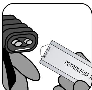
Before attaching nozzle, use petroleum jelly on face of gun. After attaching nozzle, spray into "test shot" receptacle. Unit is ready to use.
